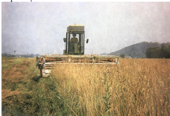
Fig. 31. Heder special montat pe un vindrover autopropulsat / Special harrow mounted on a self-propelled combine harvester
