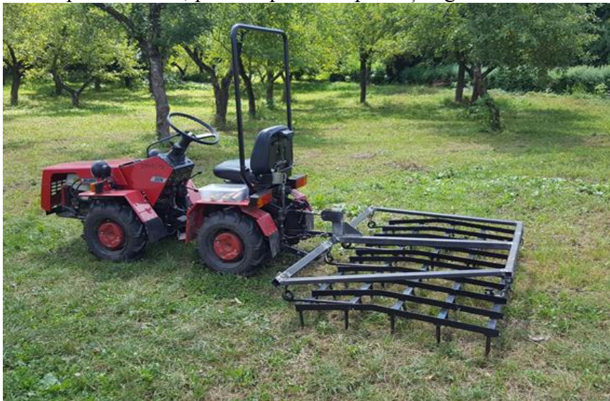
Fig. 4. Grapa cu colți fiși, tip GCF-2,0 / Harrow with rigid tines, GCF-2,0 type
