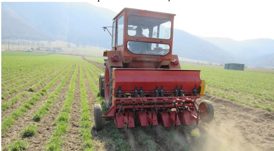
Fig. 5. Echipament de prășit și fertilizat loturi semincere, tip EPFLS-2,0 / Equipment for hoeing and chemical fertilization of seed lots, EPFLS-2,0 type.
