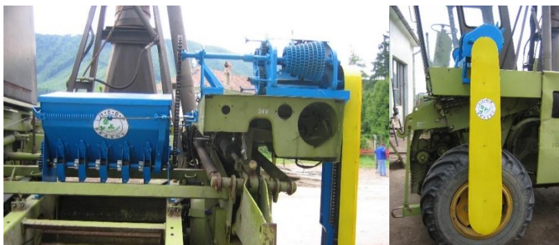
Fig. 25 Echipamentul de administrat conservant, tip EDCON / Equipment for silage additive metering, EDCON type
