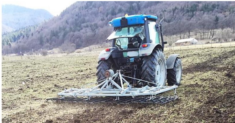
Fig. 3. Grapa cu colți fiși, tip GCF-4,0 / Harrow with rigid tines, GCF-4,0 type
